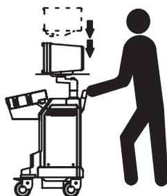
When moving the LOGIQ™ 200 PRO Series system, lower the monitor to its lowest possible position to improve stability.
